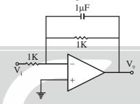
If the input is a sinusoidal wave  $V_i = 5\sin(1000t)$ , then the amplitude of the output  $V_0$  is
