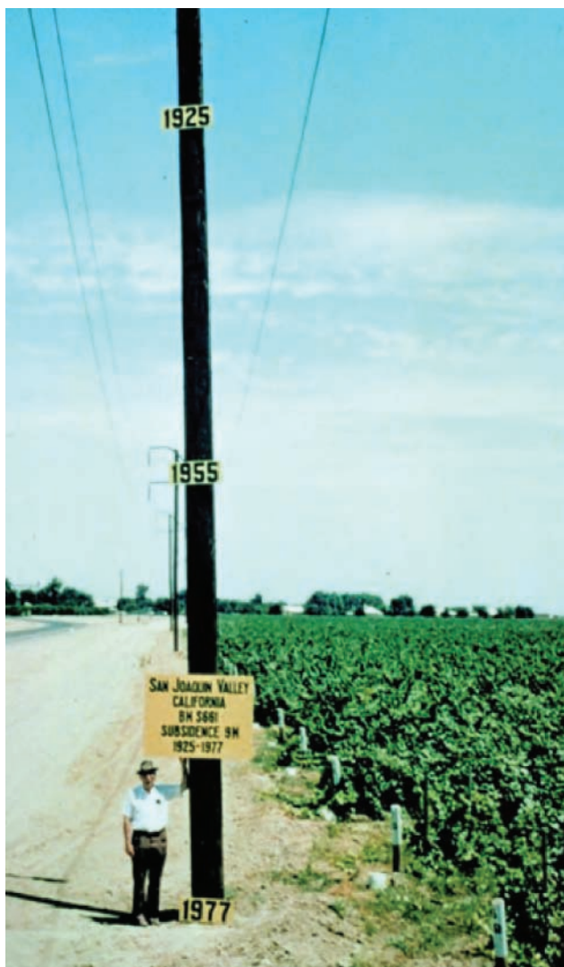
Figure 13-11 This pole shows subsidence from overpumping of an aquifer for irrigation in California's San Joaquin Central Valley between 1925 and 1977. In 1925, the land surface in this area was near the top of this pole. Since 1977 this problem has gotten worse.
