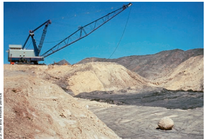
Figure 14-14 This heavy piece of equipment with a large bucket is removing material from an area-strip-mining operation in the U.S. state of Wyoming.
