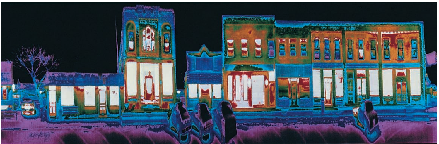
Figure 16-9 This thermogram , or infrared photo, shows heat losses (red, white, and orange) around the windows, doors, roofs, and foundations of houses and stores in Plymouth, Michigan (USA). Many homes and buildings in the United States and other countries are so full of leaks that their heat loss in cold weather and heat gain in hot weather are equivalent to what would be lost through a large, window-sized hole in a wall of the house. Question: How do you think the place where you live would compare to these buildings in terms of heat loss and the resulting waste of money spent on heating and cooling bills?
