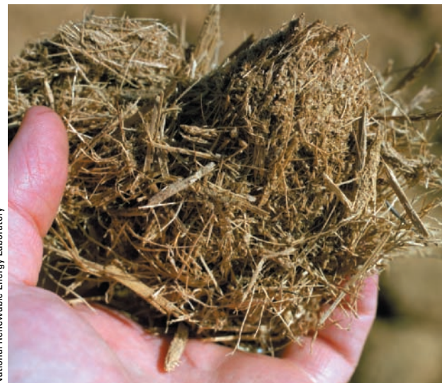
Figure 16-28 Bagasse is a sugarcane residue that can be used to make ethanol.
