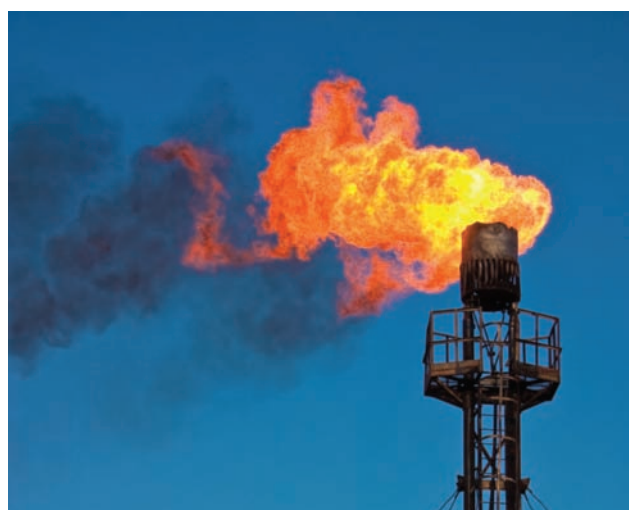
Figure 15-11 Natural gas found above a deep sea oil well deposit or in a remote land area is usually burned off (flared) because no pipeline is available to collect and transmit the gas to users. This practice wastes this energy resource and adds climate-changing \text{CO}_2 , soot, and other air pollutants to the atmosphere. Question: Can you think of an alternative to burning off this gas?
