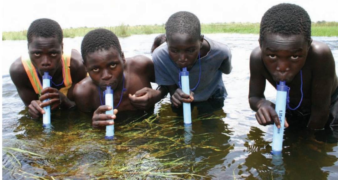
Figure 20-15 The LifeStraw™, designed by Torben Vestergaard Frandsen, is a personal water purification device that gives many poor people access to safe drinking water. Here, four young men in Uganda demonstrate its use. Question: Do you think the development of such devices should make prevention of water pollution less of a priority? Explain.
