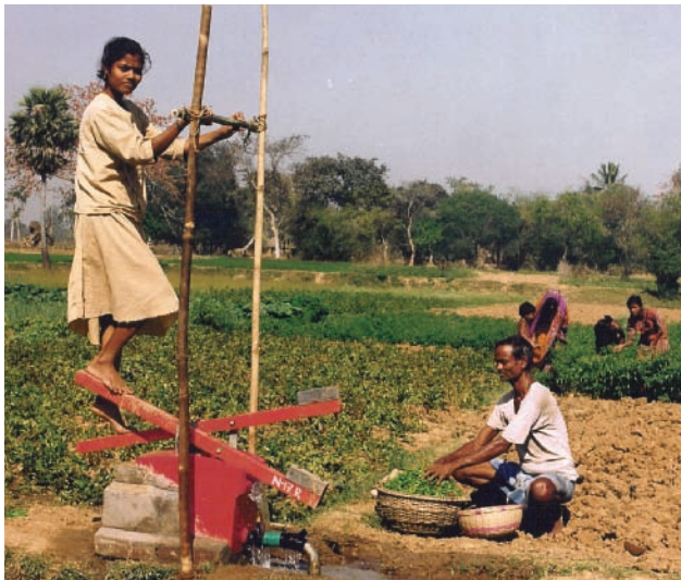
Figure 13-20 Solutions: In areas of Bangladesh and India, where water tables are high, many small-scale farmers use treadle pumps to supply irrigation water to their fields.
