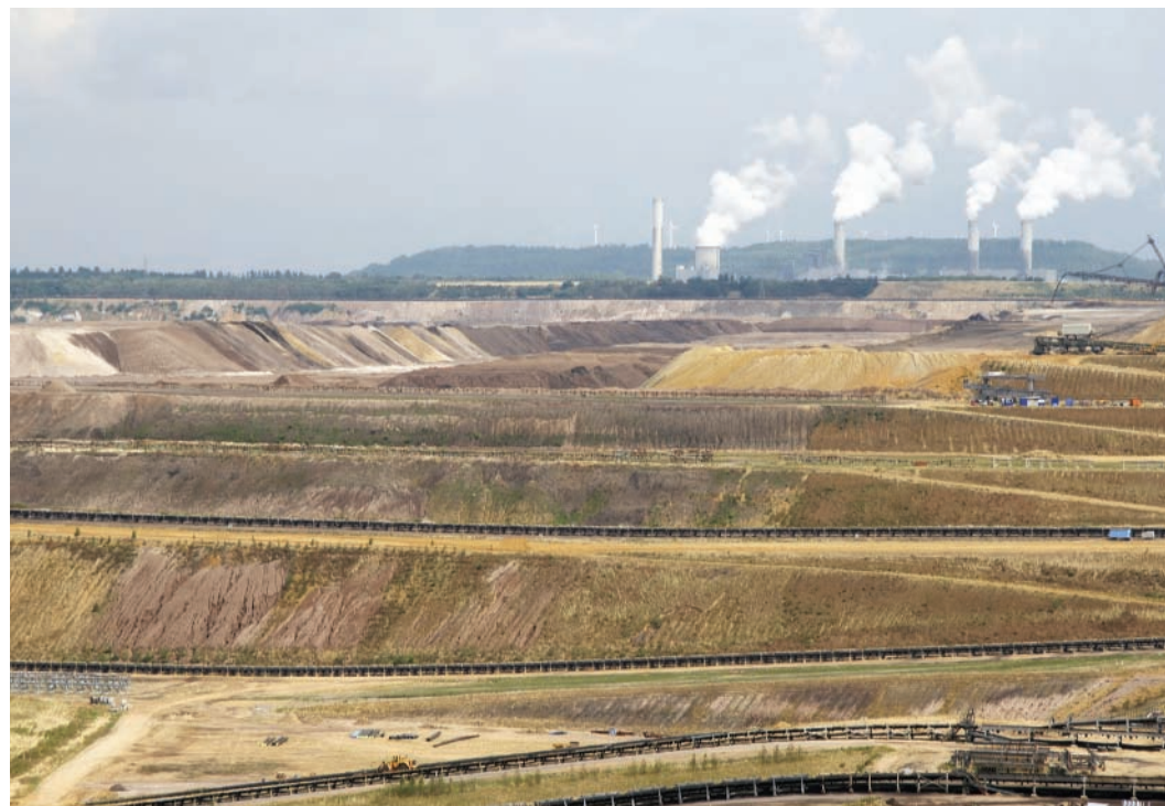
Figure 14-16 Natural capital degradation: Area strip mining of coal in Germany created these spoils banks. A coal-burning power plant is in the background. Question: Should governments require mining companies to restore such sites as fully as possible? Explain.
