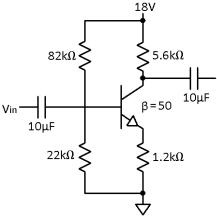
14. Determine the value of input resistance for the given circuit.
