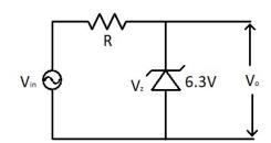
13. Determine Q point for given circuit.
